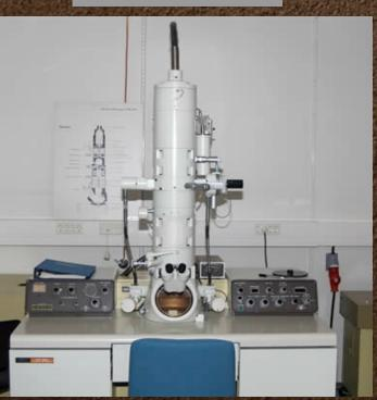
• Invented in 1931, an electron microscope is a type of microscope that uses electrons to illuminate a specimen and create an enlarged image. Electron microscopes have much greater resolving power than light microscopes and can obtain much higher magnifications. Some electron microscopes can magnify specimens up to 10 million times, while the best light microscopes are limited to magnifications of 2000 times.
